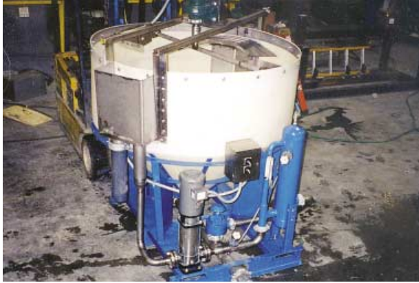
Small systems, like this Mini-DAF unit, can be supplied for flows up to 100 gpm.
